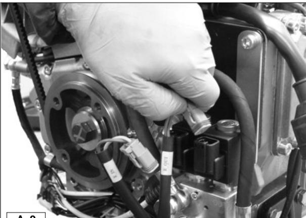
To remove connectors, press the stop tabs and draw upwards.
