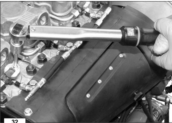
○ The fixing bracket screws must be tightened to 10 Nm using a torque wrench.
