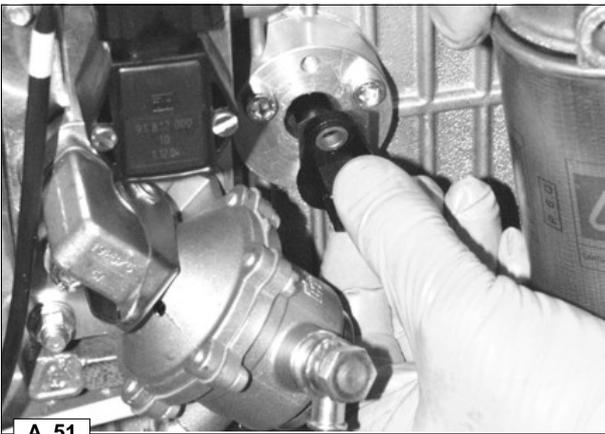
Remove the sensor from the support taking care not to damage the O-ring.
