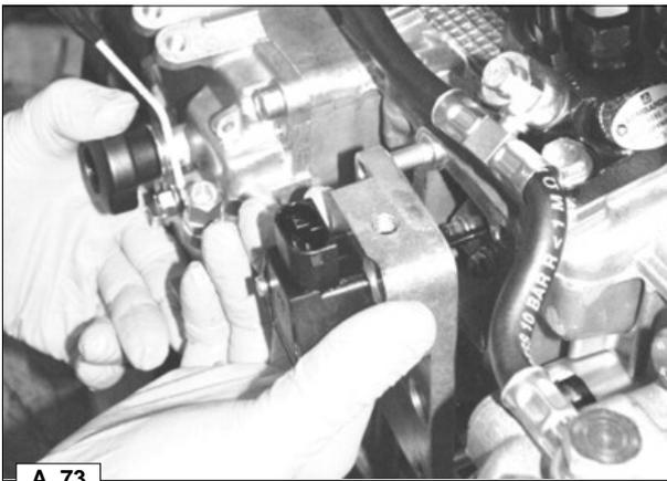
Look through the upper inspection hole on the cover to make sure that the pin 1 is correctly inserted into the fork 2.
