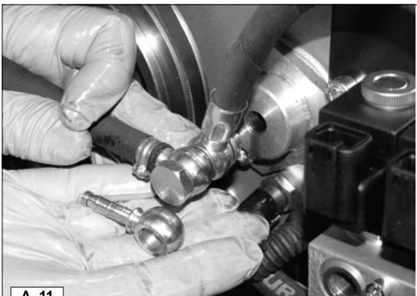
On the opposite end of the block of pipe 19 is the variator lubrication jet attached to the pipe by a click clamp.
