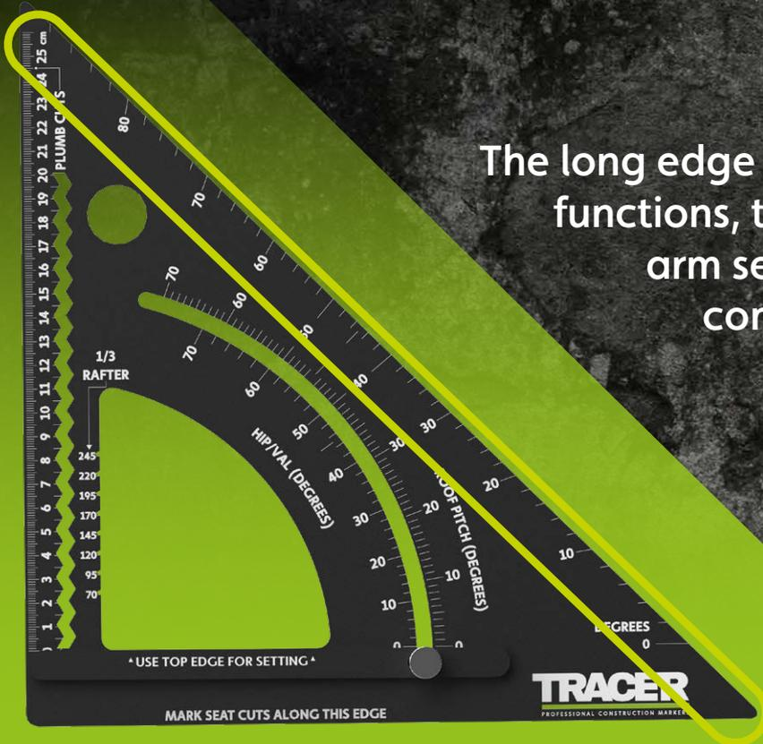
The second, like the set-square, is the ability to quickly create an angled mark. Just pivot the square using the graduations on this outer edge as a guide. You can now quickly and simply pivot the square to mark any angled cuts from 0°-90°.
