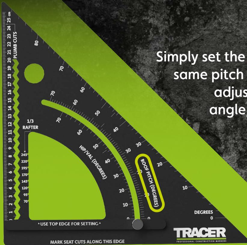
Simply set the TRACER ProSquare to the same pitch of the roof by moving the adjustable arm to the required angle, lock it off. Once the roof pitch measurement is set the angle will be correct for both the Seat and Plumb cuts.
