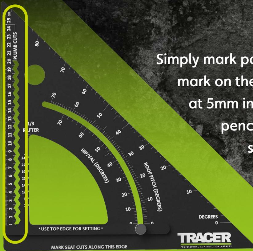
Simply mark parallel lines with the 'parallel' mark on the side of the square – marked at 5mm increments, simply locate your pencil in the necessary depth and slide along the desired length of your timber.
