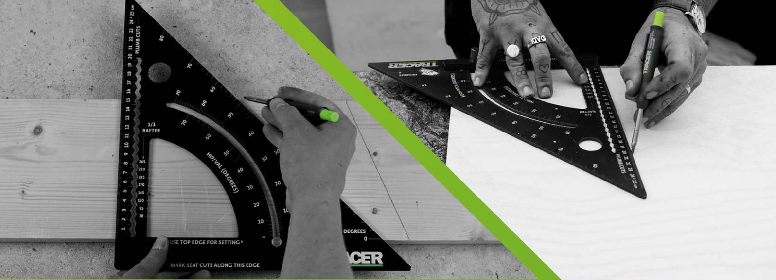
"Very simple to use. Just need to set the scale to whatever the roof pitch is and mark your seat and plum cuts for either the Jack and Com or Hip and Valley cuts!"
