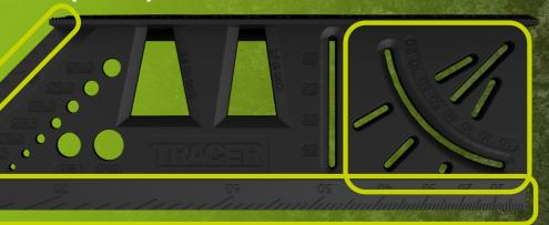
Large, detailed 0-90° protractor along the outside edge, the most convenient way to mark on an angle. This face also includes a smaller detailed protractor 10-80° with a pre-set of 30,45,60° markings.
