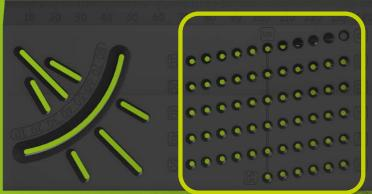
With measurement going up in 1mm increments simply select the correct depth hole, insert a sharp pencil, and run the mitre tool down your material for the desired depth/length!
