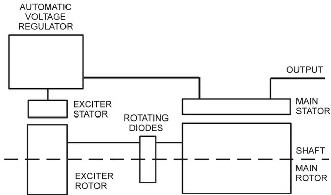
The main stator provides power for excitation of the exciter field via the SX460 (SA465) AVR which is the controlling device governing the level of excitation provided to the exciter field. The AVR responds to a voltage sensing signal derived from the main stator winding. By controlling the low power of the exciter field, control of the high power requirement of the main field is achieved through the rectified output of the exciter armature.
