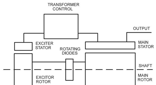
The main stator provides power for excitation of the exciter field via a transformer rectifier unit. The transformer combines voltage and current elements derived from the main stator output to form the basis of an open-loop control system, which is self regulating in nature. The system inherently compensates for load current magnitude and power factor and provides short circuit maintenance in addition to a good motor starting performance.
