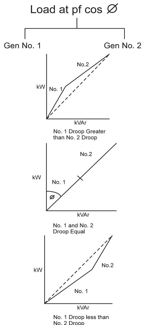
Generally 5% droop at full load current zero p.f. is sufficient to ensure kVAR sharing.
