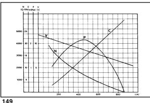
Characteristic curves for starting motor type Magneti Marelli E100, 1.5/12 V
