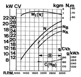
N (DIN 70020)Automotive rating, intermittent operation with variable speed and variable load. NB (DIN 6270)Rating with no overload capability, continuous light duty operation with constant speed and variable load. NA (DIN 6270)Continuous rating with overload capability, continuous heavy duty with constant speed and constant load.
