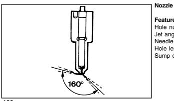
Features: Hole number and diameter 4x0.28 mm. Jet angles =  $160^{\circ}$ . Needle valve elevation = 0.20 ÷ 0.22 mm Hole length = 0.7 mmSump diameter and length = 1x1.5 mm
