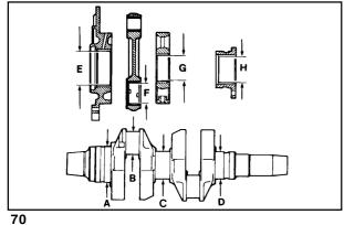
Clearance between main journals/crank pins and connecting rod bearings (mm)
